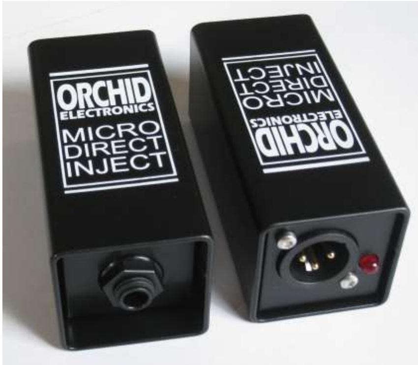
Housed in a strong steel tube 90 X 40 X 40 it has only a jack socket input for connection to the instrument and an XLR output to feed the microphone input of a mixing desk - which can be located many hundreds of metres away if necessary. It must receive Phantom Power from the mixer as it is an active design - a red LED will indicate power present.
