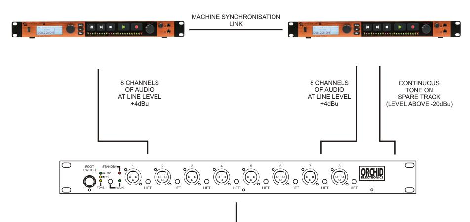
IN AUTO MODE - UNIT SWITCHES TO MAIN MACHINE WHEN THE TONE IS DETECTED
